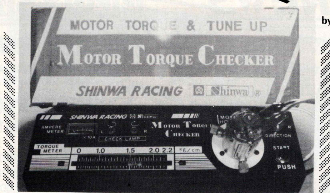
The Shinwa Torque Checker provides a quick and easy torque reading of the RC electric motor. The reading is shown on the scale in Kg-cm. In this photo the Yokomo 05R under test has an output torque of 1.6 kg-cm.
