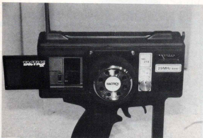
A panel slides out on the left of the transmitter to reveal the servo reversing switches.
